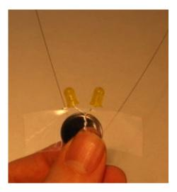
Now wrap each tape wing around the bottom (negative) side of the battery, firmly taping the twisted LED leads in place:
