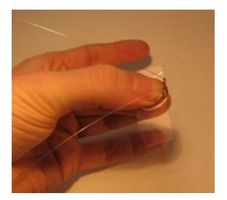
Now grab the LED eye assembly. The twisted-together LED leads will be taped to the negative side of the battery, with the eyes facing forward—the same direction the
