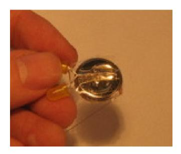
Now pick up the leg assembly and carefully place it onto the battery so that the point at which the pipe cleaners are twisted together meets the glob of glue:
