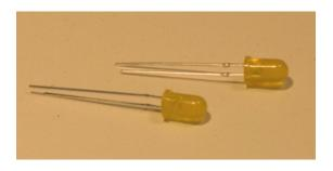
Notice that each LED has 2 wire leads, and that one lead is slightly longer than the other. The long lead is the "positive" lead... this is important, as LEDs need to be oriented the right way, or they don't work!
