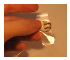
Use your fingers to work the tape into the nooks and crannies around the copper tube, but let the tape wings to continue to extend of either side of the battery.
