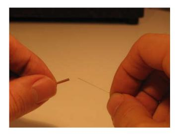
Slide the tube about ½ of the way down the length of the wire. Use the ruler to help center it; there should be 5 ¾" of wire extending from either end of the tube. You use a little piece of tape to help keep the wire in place, like so:
