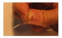
In the above photo, the tape is on top of the base of the copper tube, with the sticky side down. Next, lay this antennae/tape assembly on top of the positive side of the battery:
