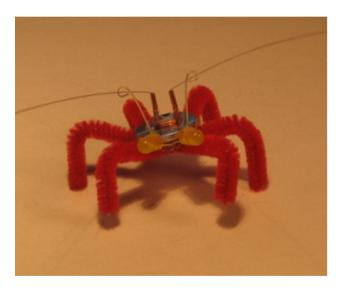
When an antenna is moved slightly, it contacts the loop and turns that eye "on:"
