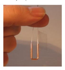
If one section of copper tube is slightly longer than the other, don't worry about it... this is not an exact science! You can now remove the bit of tape. Here is another view of what we have so far (don't worry if the wires cross like this or not):
