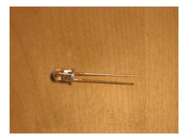
The longer lead is the "positive" lead (this will be important later). Now gently bend the positive lead about 15 degrees:
