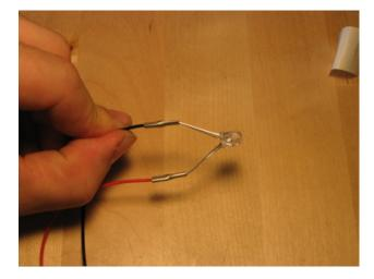
It is very important that the two splices never touch, if they do, it will prevent your LED Art from lighting up, and quickly drain the battery.
