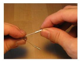
Again, give it a good squeeze, being careful only to crimp the LED side of the splice:
