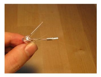
It's very important that you remember which are the positive LED leads; you may want to mark this splice with a small piece of tape. If you get confused, each LED lens has a little flat spot next to the negative lead.
