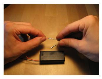
With your pliers, squeeze the splice firmly over the red wire:
