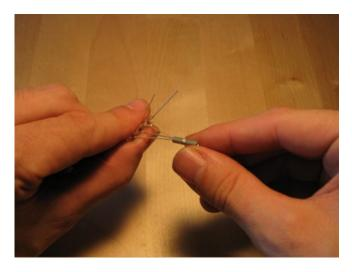
With your pliers, squeeze the butt splice where it encloses the 3 LED leads, being careful not to crimp the opposite site of the splice. Apply enough pressure so that the 3 leads are held solidly in place:
