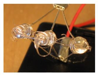
Let the glue cool, and see how it looks when projected against the screen. Give it a few minutes to let the LEDs cycle through their various colors. Feel free to experiment, as it's easy to peel the cooled glue off the lens and try something different!
