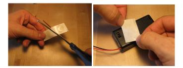
Press firmly, and peel off the backing (if needed, use your finger to help the glue dot stick to the case, but try not to touch the glue more than necessary):
